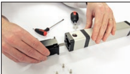
Insert motor shaft into coupling
