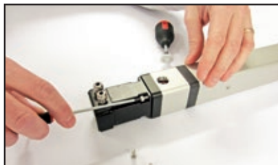
Tighten motor mounting screws
